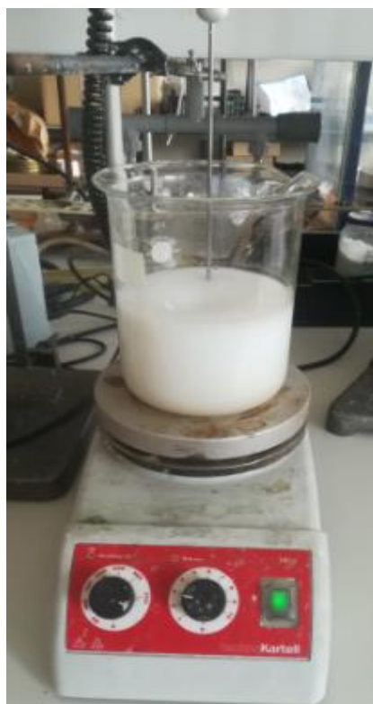
Fig. 13 Magnetic stirrer used for preparation of HT
