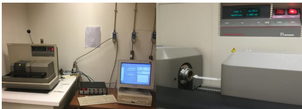
Fig. 16: TA Instruments SDT 2960 simultaneous TGA/DSC apparatus with computer and samples.
