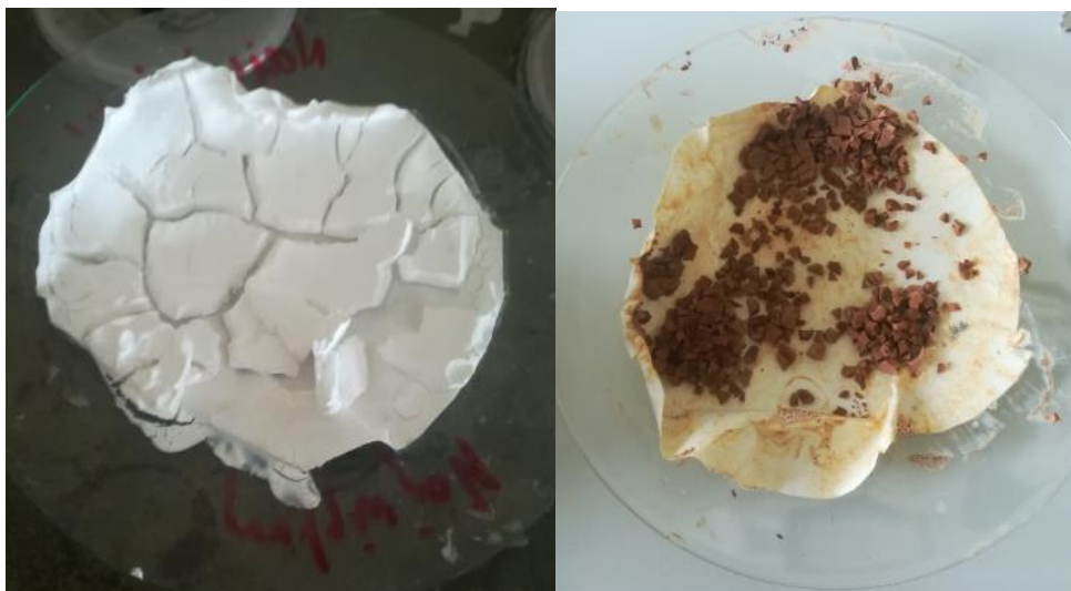
Fig. 15 Hydrotalcites obtained through co-precipitation method after being dried – Zn/Al (left) and Mg/Al.Fe (right)
